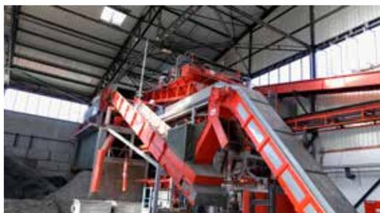
**3** A Pyrosmart system monitors the falling flow at the conveyor belt downstream of the shredder at Jakob Becker Entsorgungs-GmbH. In the event of a fire, the material is redirected to a special fire box, averting a fire
