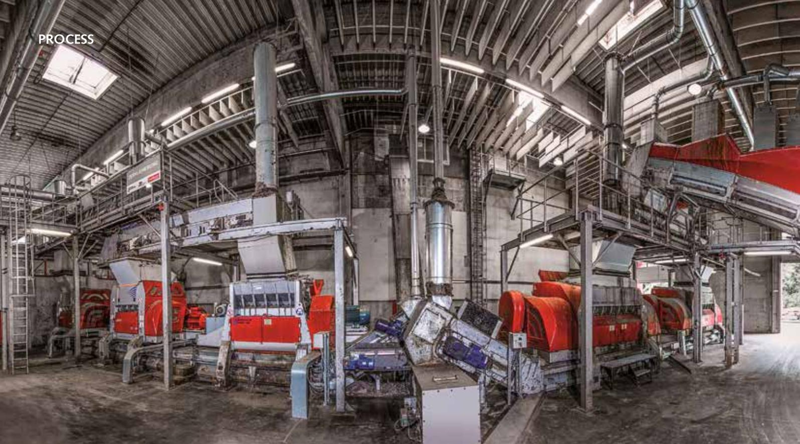
**2** The plant at the Austrian company ThermoTeam Alternativbrennstoffverwertungs GmbH crushes the material with shredders and separates unwanted components, such as metal and inert materials
